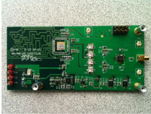
Figure 2 Waveform synthesizer with up-conversion for radar waveform generation.
